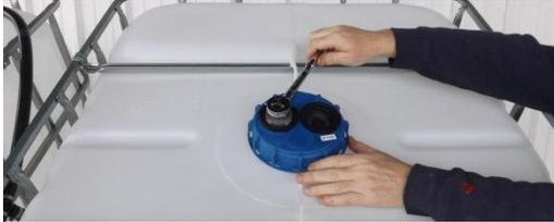
B - Tighten valve as required.
