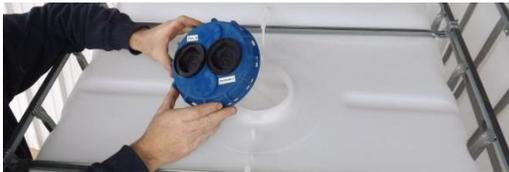
B - Replace the caps you just removed with the 6" IBC caps that have the 4 Cam dispense valve and 4 Cam fill valve factory installed.
