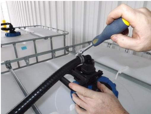
With the existing dispense coupler properly installed; affix the hose from the manifold assembly to the barbed fitting by using the supplied hose clamp. The proper end of the hose is identified with a yellow tag.
