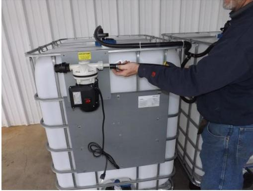
Attach the open end of the hose that is affixed to the bottom of the “T” fitting in the center of your hose manifold to the suction side of your pump.
