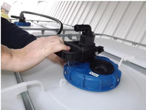
Install your existing dispense coupler to the 4 Cam fill valve previously installed in Step 8. (Note: You will need to remove the existing hose from the coupler and pump at this time.) When properly installed, your existing dispense coupler should be aligned in manner consistent with the installation completed in Step 5.
