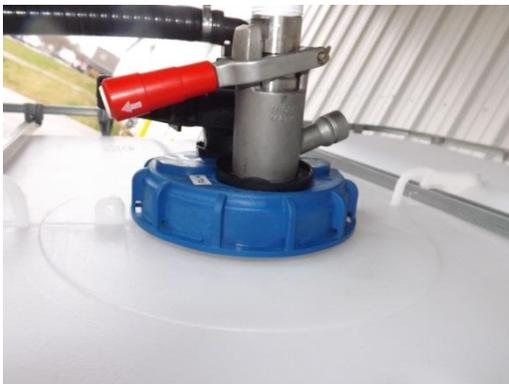
When the dispense couplers are properly installed, a fill coupler can be affixed to the fill valve(s) as shown.
