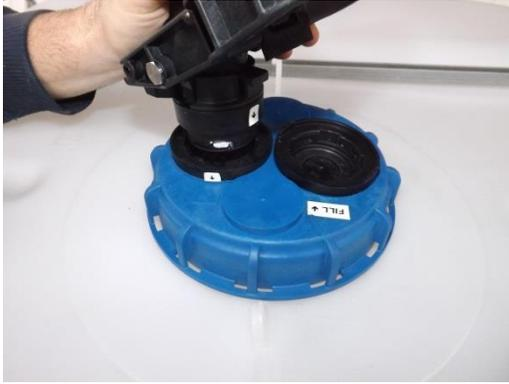
Your manifold hose assembly comes with two 4 Cam dispense couplers factory installed. (One dispense coupler will be installed on the end totes.) Align the white cam on the coupler with the arrow on the valve's collar.
