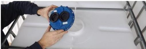
B - Replace the cap you just removed with the 6" IBC cap that has the 4 Cam dispense valve and 4 Cam fill valve factory installed.
