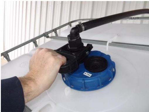
Depress the coupler handle so that it is in the locked position.
