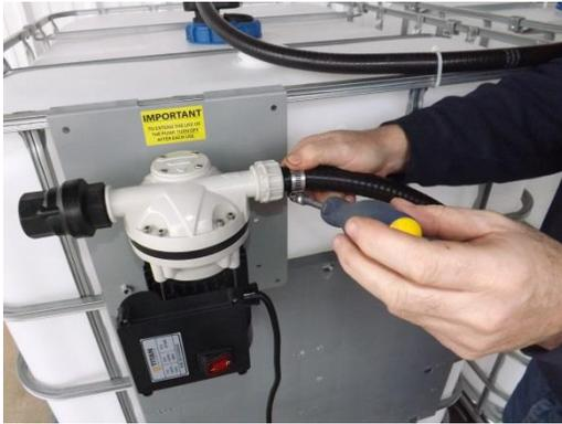
Tighten the hose using the hose clamp provided.
