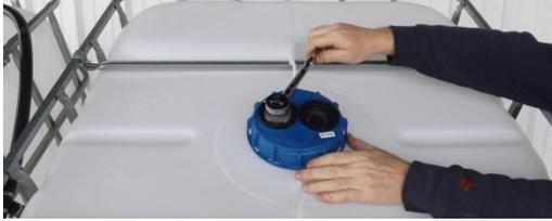
B - Tighten valve as required.
